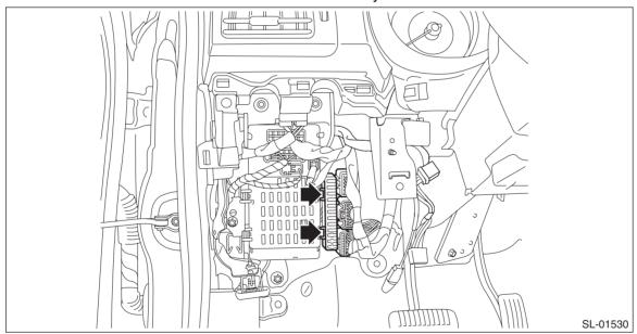
4) Disconnect the connectors from the relay & fuse box.
