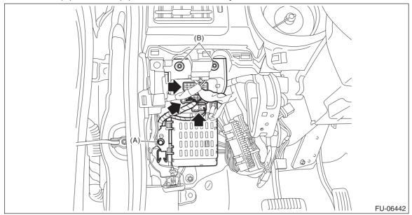
6) Remove the electronic throttle control relay from the relay block on the back side of the fuse block.
